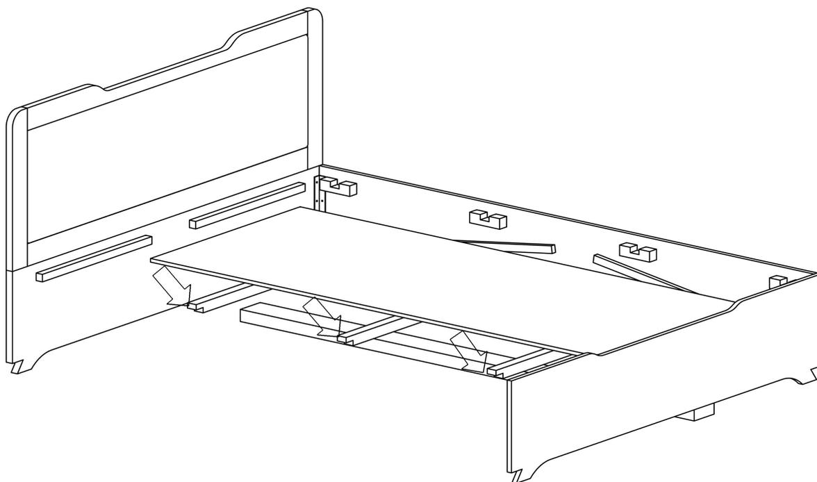
Now Place Part-G(Bottom Panel) into last assembled part as shown in fig.
