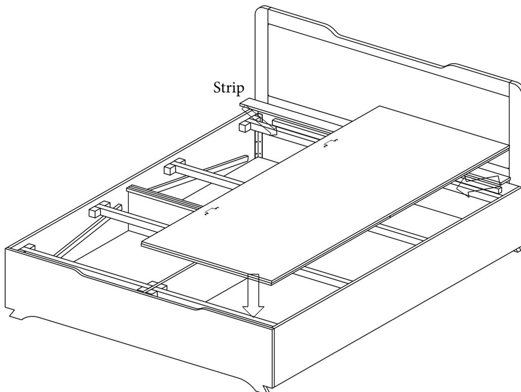
Now place Part-B (Top strips) and Part-I (Top panel) at last assembled as shown in Fig.
