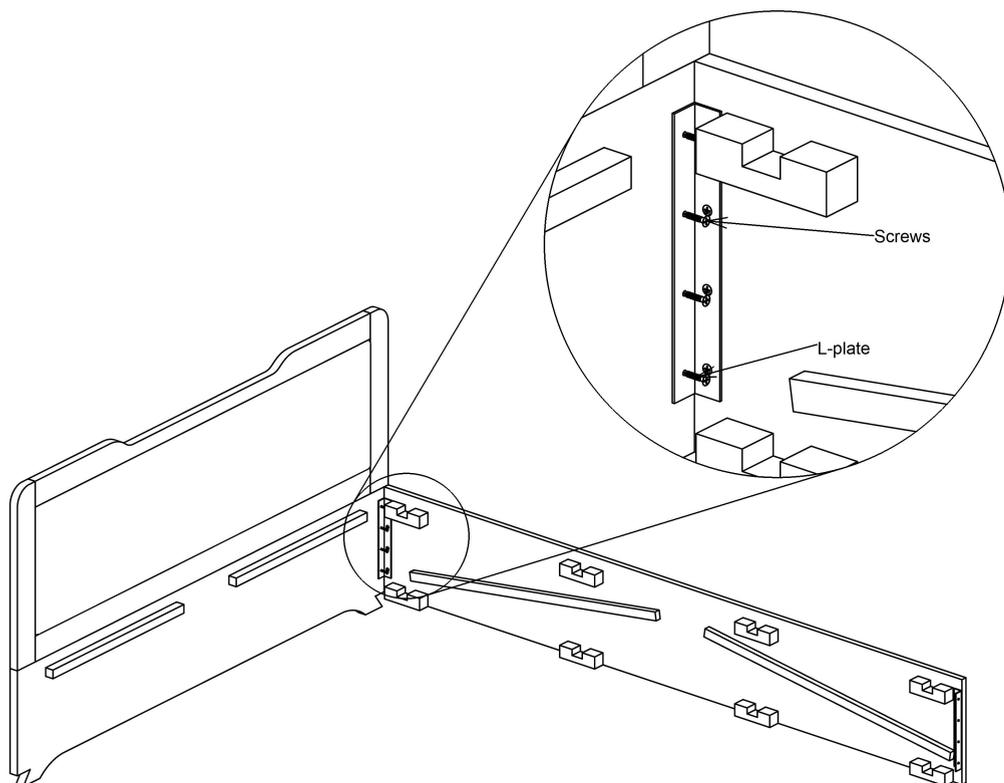
Fix the Part -A(Headboard) and Part-C(Sideboard) on using L-plate with the help of Screw 16mm as shown in fig.
