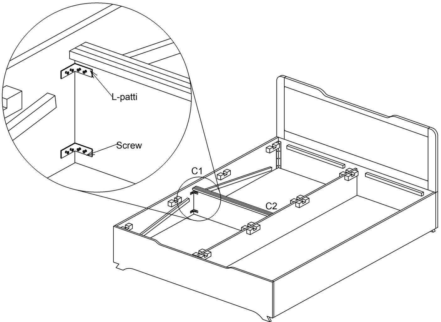
Fix the Part -F(Middle partition) with last assembled part using l-patti with the help of screw at defined position C1 and C2 as shown in Fig.
