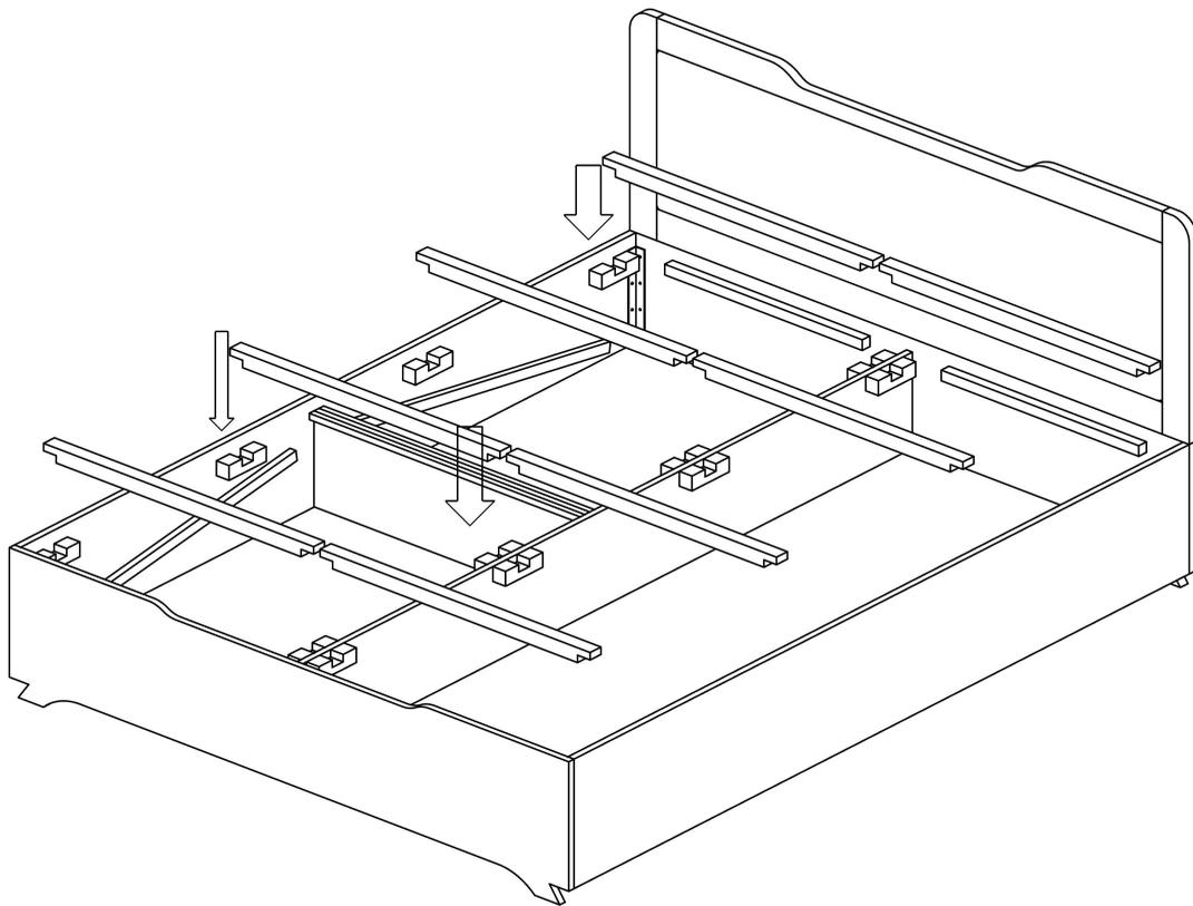
Now fix Part-E (Battens) at upper U-block as shown in Fig.
