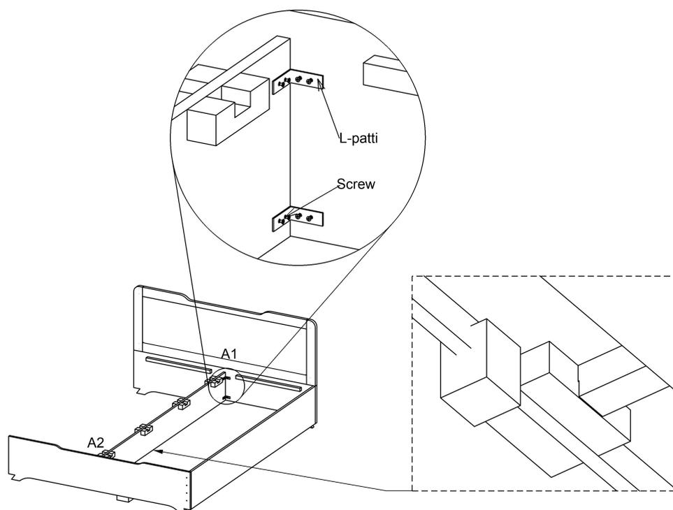
Now place battens in U-block of Part-D(Middle panel) and fix Part -D with Part- A (Headboard) and Part-H(Footboard) by L-patti and screws 16mm at position A1 and A2 respectively as shown in fig.
