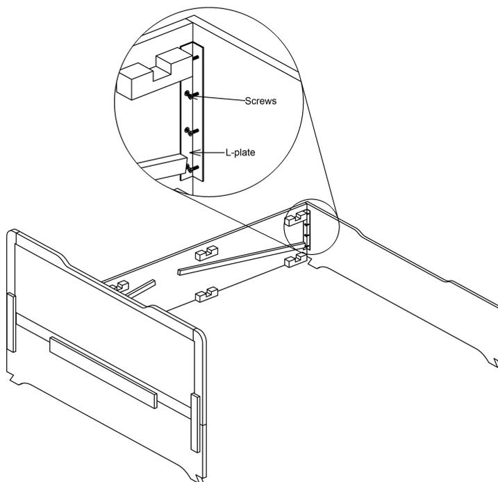
Fix the Part-H (Footboard) and last assembled part with L-plate and screws as shown in fig.
