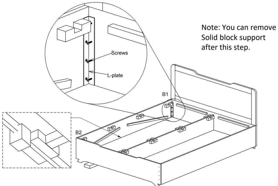
Now place battens in U-block of Part-C(Side panel) and fix Part -C with Part-A (Headboard) and Part-H(Footboard) by L-plate and screws 16mm at position B1 and B2 respectively as shown in fig.
